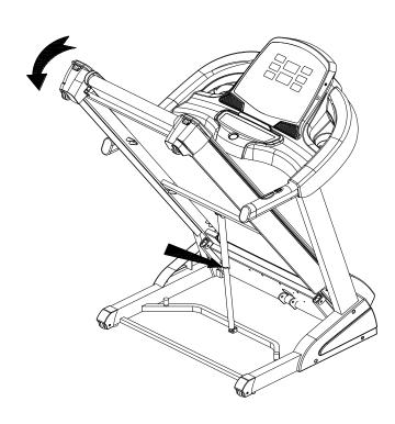
Lightly push the rear of running deck, and kick gently the cylinder also press the rear end of treadmill in the meantime to let it unfold slowly.
