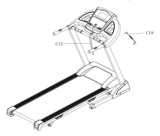
**Step 6:** To check if the running belt runs correctly, placing treadmill in folding position and tightening all the bolts. Then set speed under 3km/h and see if running belt runs without problem.
