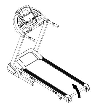
Lift up the machine and force to pull up until you heard "click" that made by safety casing stuck the pneumatic cylinder.
