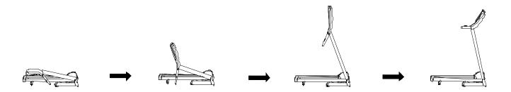
**STEP 3:** According to the picture, tighten the bottom frame with bolt M8\*45(D16) and inner washer(D17). Then locked the console frame with M8\*15 (D13) and inner washer (D17).
